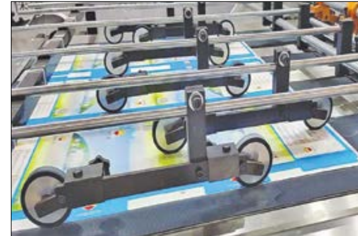
Collection and delivery table both adopt the vacuum inspiration to avoid the problem of the gripper biting no paper. The device applies to common paperboard, E/B/A corrugated paper and plastic board.
