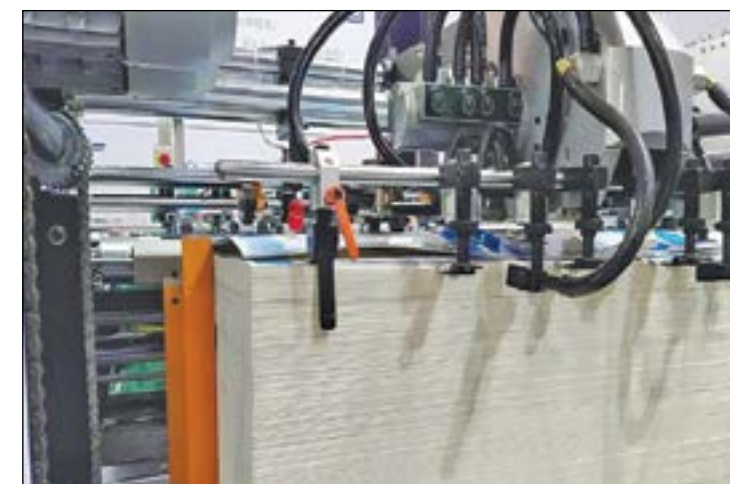
The feeder part is equipped with track device, separating freely when you make plate.
