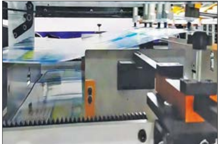
The front block and side block can adjust freely in accordance with the paper size. Easy to adjust and precisely.
