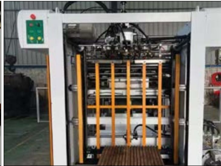
Delivery table is equipped with automatic support device. Continuous operation without stop, works efficiently.
